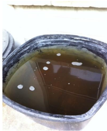
Fig. 2. Curing tank filled with 100 times dilution of EMC
