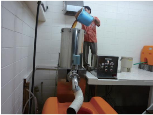
Processing the same amount of food waste and Activated EM • 1 Crush approx. 100L of solid waste for 10min
